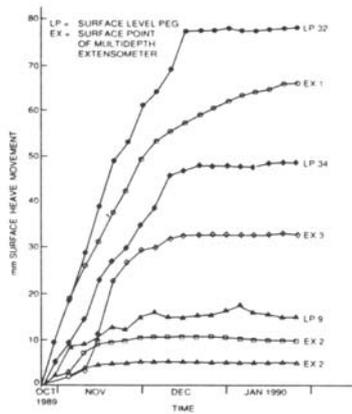
*Time – Surface Heave Relationship Following Flooding. Blight et al, (1992)*
